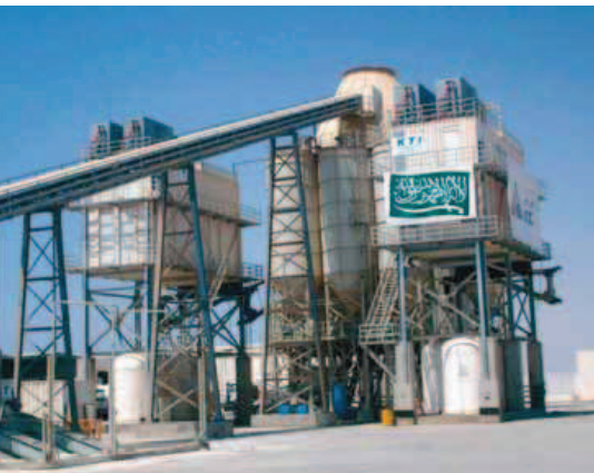
Ice plants have been built in the gulf to keep concrete protected from high temperatures.
